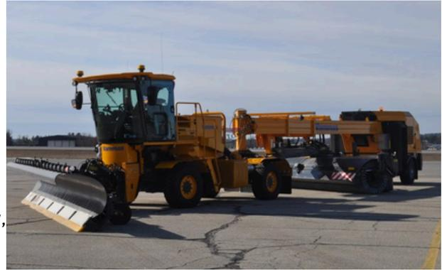
The Vammas operating system is fully automatic, initiating all systems based on the operator's selection within 8 seconds. The Aggregate engine will increase or decrease based purely on the joystick selection, saving fuel during operations.
