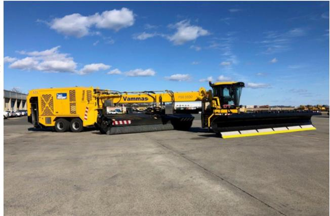
Vammas PSB 5500 units have combined front wheel and rear articulated steering, to effectively maneuver on airport taxiways, aprons and runways. With the capability of operating at 37MPH (60 KM/H), the PSB 5500 minimizes runway occupancy times and keeps your airfield open longer.
