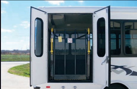
Optional double wheelchair door with top mounted gas shocks to hold door open in windy conditions
