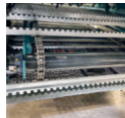
Pick-up blade with transport system unit
